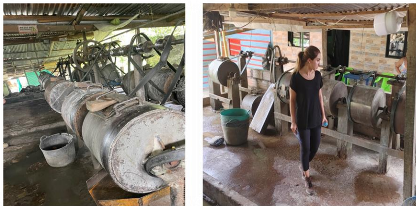
Figure 2-3. Small ball mills,” Cocos”, in an urban processing center, Providencia, Colombia.
